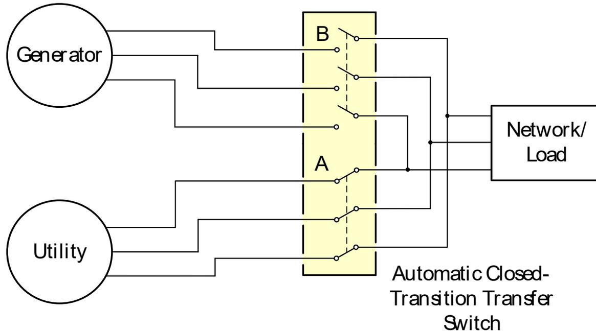
1. Diagram shows 'overlapping' contacts but usual arrangement is two independent sets of 3 or 4-pole contacts (Switch A & B)....
