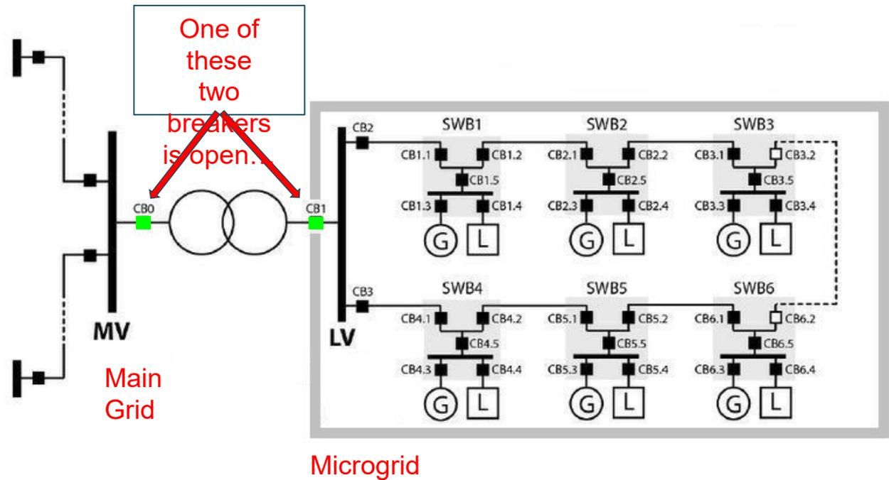
Creating a microgrid 'island' upon a main grid failure is relatively easy *if* the conditions for sustained operation exist at the moment of failure ....
