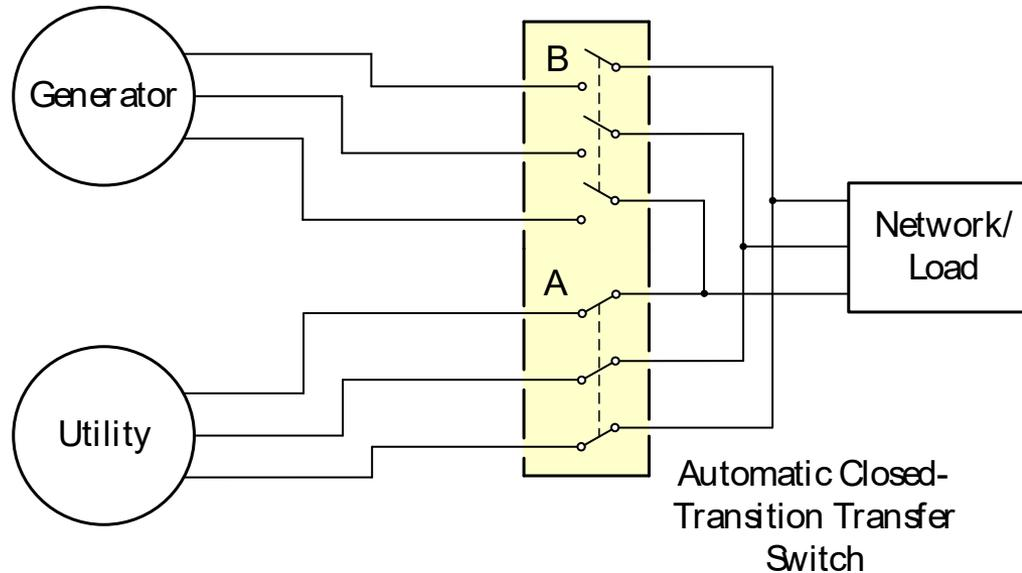
4. Typical operation of a closed transition ATS:
